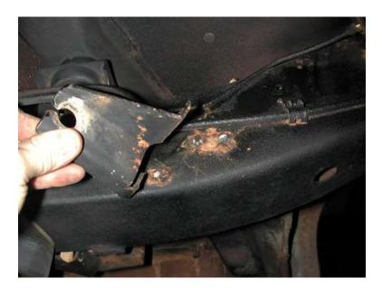
3. The parking brake brackets will be in the way of the 4 link and must be removed. Loosen the parking brake adjustment nut and remove the cable from the frame bracket. The tack weld can be broke loose with a hammer and chisel. Grind the remains of the weld smooth.
