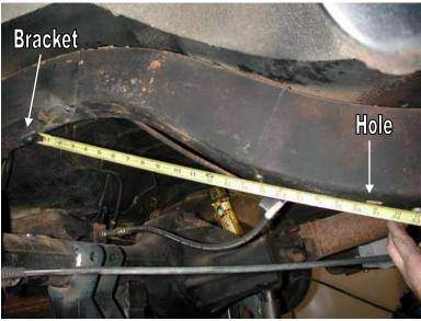
6. The location of the upper Shockwave mount is determined by measuring 14 ½" from the edge of the bracket to the large hole in the bottom of the frame.
