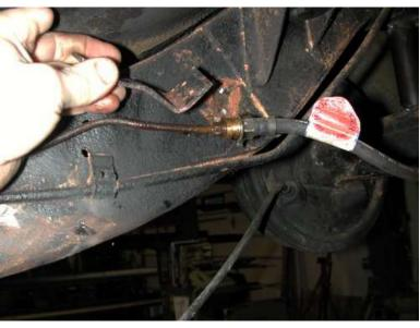
4. The rear brake line bracket on the passenger side fame rail must also be removed. Be careful not to cut fuel line.
