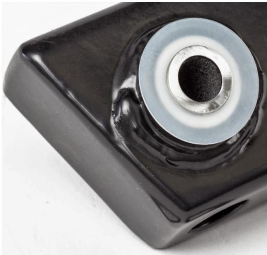
PLEASE NOTE : The thin Nylon washers help hold the grease inside the bushings keeping them lubricated. For Maximum life, the Delrin bushings must stay lubricated frequently with a synthetic grease.
