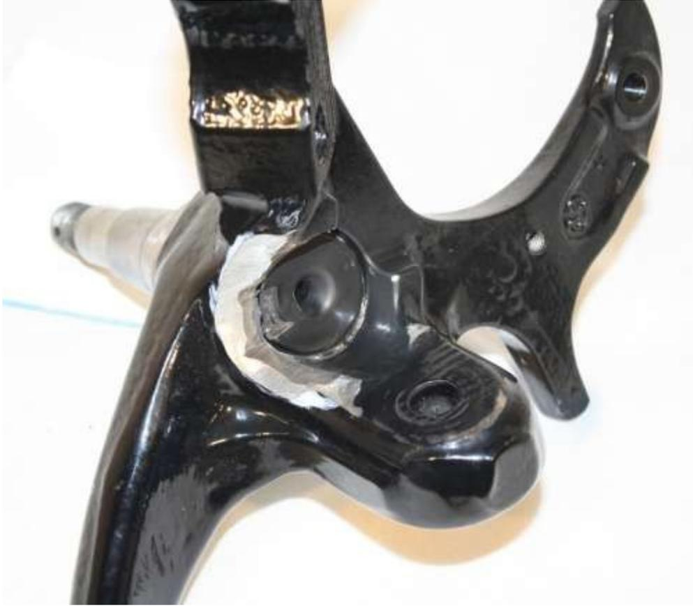
**Clearance Required On Top of Heavy Spindles For Bolt Alignment**
