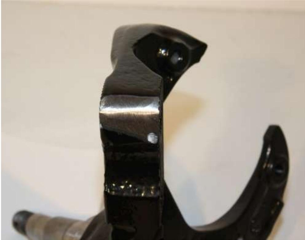
**Finished: We Have Now Gained The Clearance Needed To Mount The Strut**
