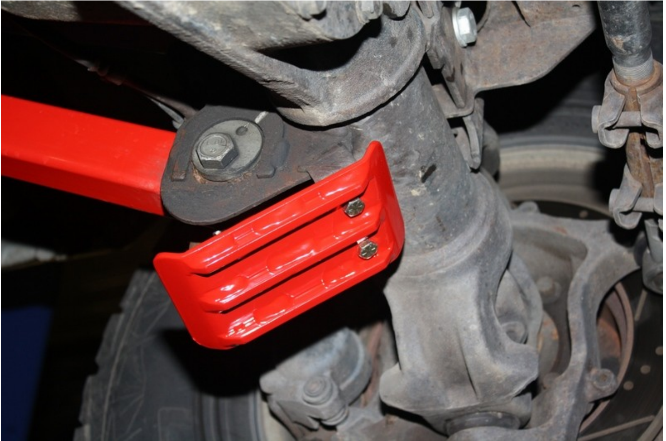
Spohn Performance front lower control arm skid plate installed
